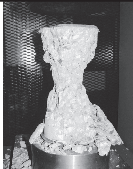
Fractured Test Specimen at Failure
